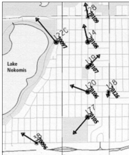
Figure B.1. Portion of a Minneapolis control quality map identifying the magnitude and direction of differences between city monuments and corresponding vendor-supplied data.
