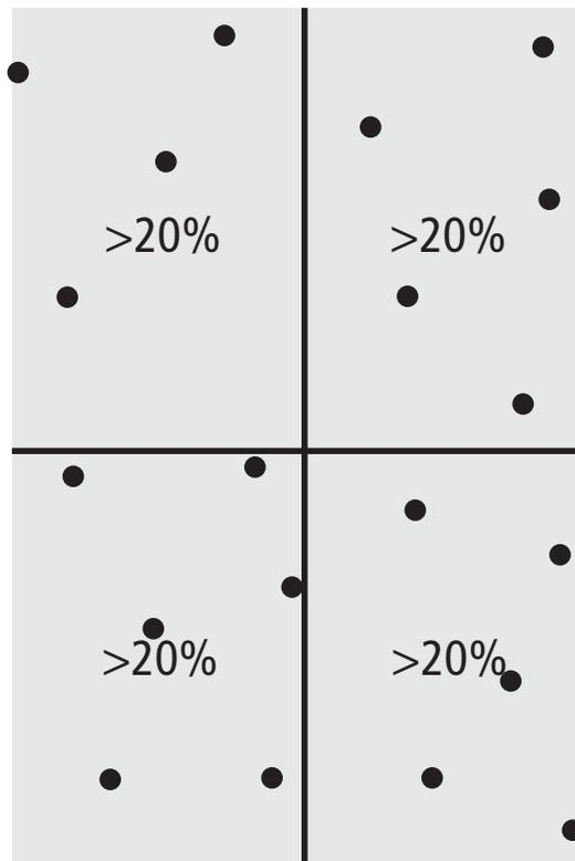
**Figure 3 (right).** Ideal test point spacing.
